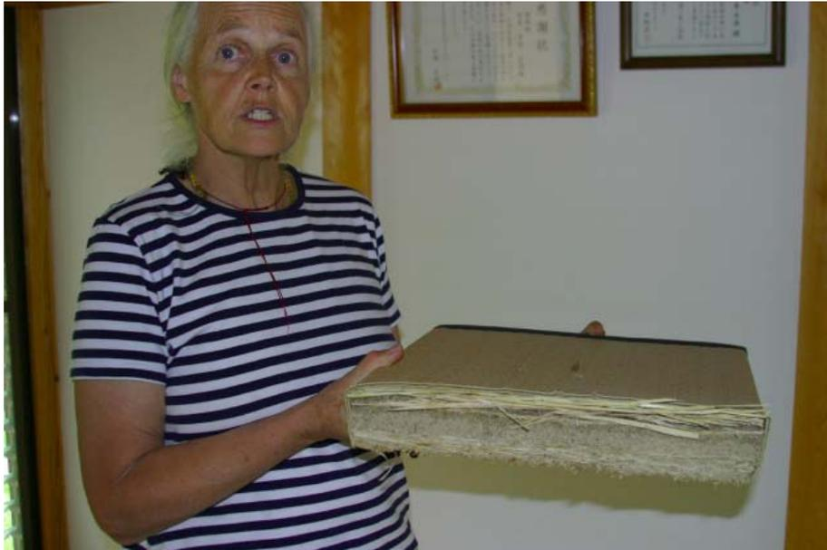
Tatami floor mats sample cross section typical of those widely used in Japan with recycling potential
