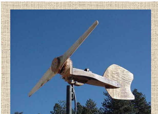
self-build: this 300W wooden wind generator was made from scratch (including the alternator!) at minimal cost using only wood, copper wire and surplus computer hard drive magnets.
